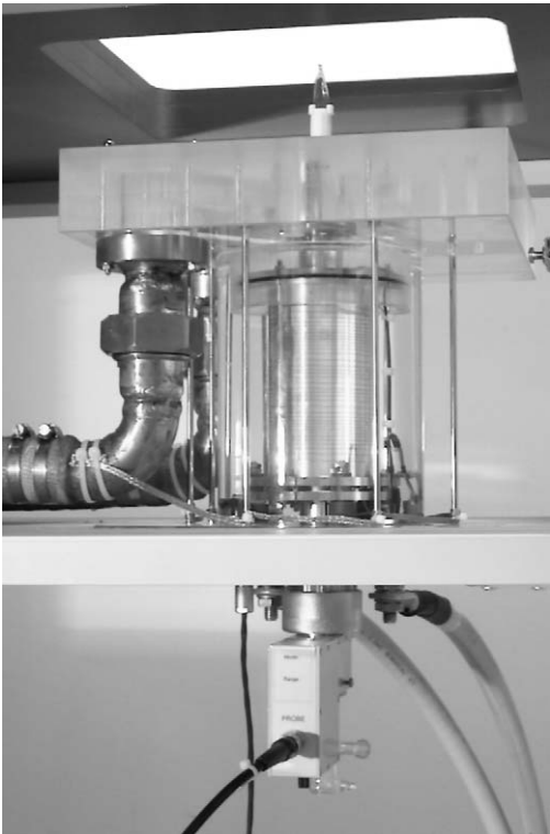
FIG. 8. The 1 T magnet assembled inside its enclosure.
